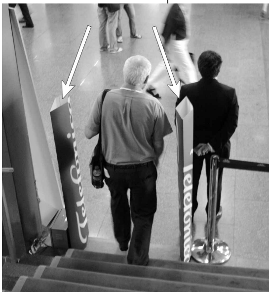
(top) RFID tags stuck to conference badges monitor attendance. (bottom) These twin pillars are RFID readers.
